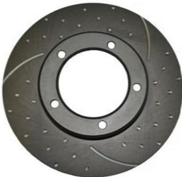
Figure 3 Disk of slotted type
