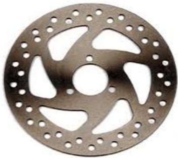
Figure 2 Disk of drilled type
