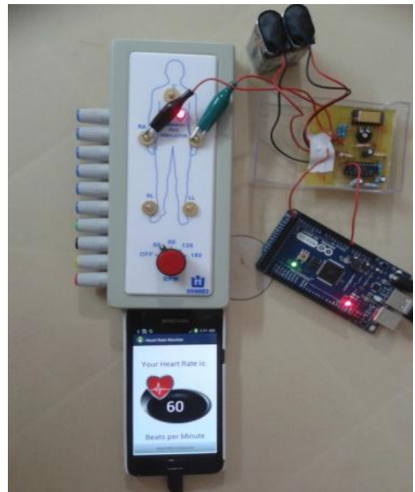
Fig.7 A: The Heart Rate set by the ECG simulator displayed on the phone application
