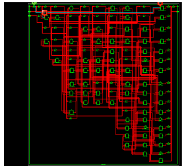
Fig.9: Technology Schematic of 16bit-BK-BEC Carry select adder
