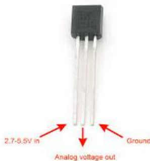
Fig: 4. Temperature Sensor
