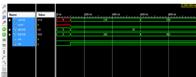
Figure 7: Simulated output for 16 bit PASTA adders
