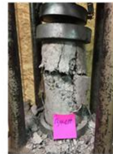
Figure 4-2 Cylinders failure pattern
