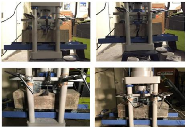
Figure 4-9 Failure stages of plain concrete
