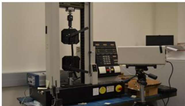
Figure 3-5 Direct tensile testing machine “Instorn”
