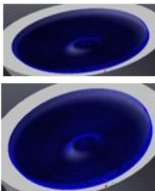
**Figure 4.3 Tool path with 0.10 mm step over**
