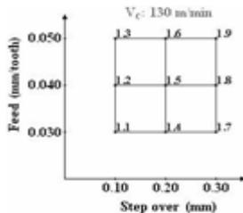
**Figure 5.1 Design matrix for the first set of experiments**
