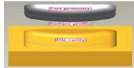
**Figure 5.14 Die and forging part geometries for the case s**
