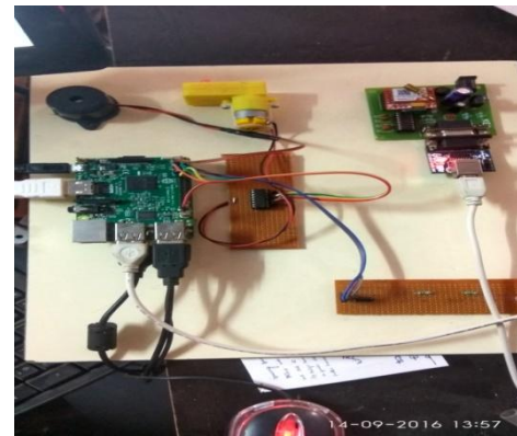
Fig10. Topview of hardware design showing Raspberry Pi board, GSM module, IR sensors, buzzer and DC motor
