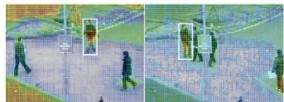
The classifier response (heat map) visualized for one tracking target (white). As the classifier is adapted continuously, it becomes more discriminative (right: 20 frames later)
