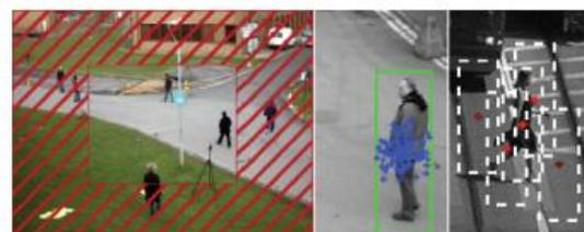
The initialization and termination region for a typical surveillance scenario (left). The initial particles are drawn from a normal distribution centered at the detection (middle). The weight of each particle is determined by evaluating the respective image patch (right). During tracking, they decrease inversely proportional to the number of successfully tracked frames (down to a lower limit). Hence, the longer a target is tracked successfully, the less the particles are spread.
