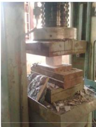
Fig. 4.10 Determination of compressive strength of cube
