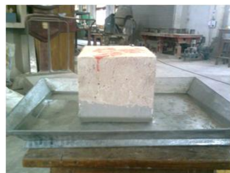
Fig. 4.24 Capillary absorption test of cubes
