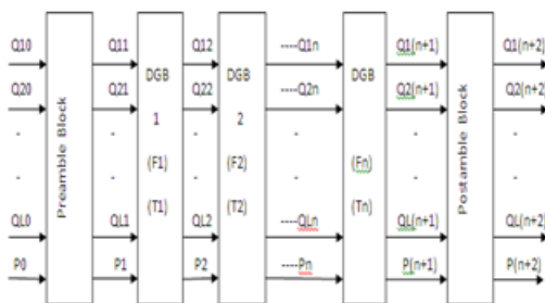
Fig. 7. Block Diagram of Online Testable Reversible Circuit
