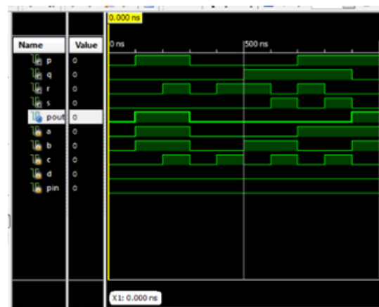
Figure -13. Simulation results of Single Missing Gate Fault in original gate.
