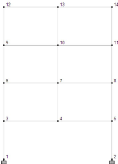
Fig.4.2 2D Frame with Floating column
