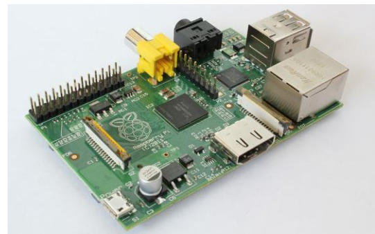
The Raspberry Pi has a Broadcom system on a chip (SoC).
