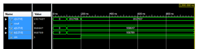
Fig.10: Simulation of 128-bit reversible carry look-ahead adder
