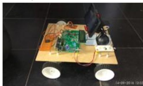
Figure 5. Sideview of the AndroRC shows the android device as camera, DC Motors, ARM 7 board, and Wi-Fi router.
