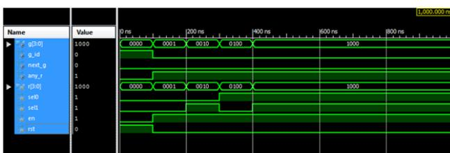
**Fig10: Simulation output waveform of an Index-based Round Robin (IRR) arbiter.**
