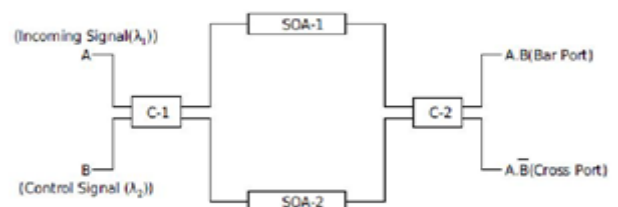
Fig.2.SOA based Mach-Zehnder Interferometer switch [8]
