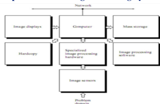
Fig.1.4. Components of a general purpose Image Processing System
