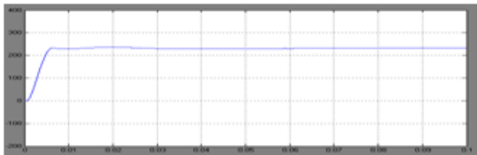
Figure 15: Converter DC voltage under operating condition using PWM
