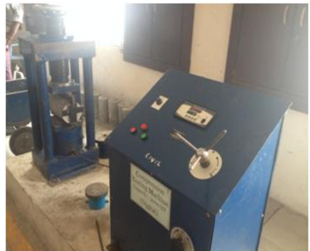
Fig 3.1.3 Split tensile set up in CTM
