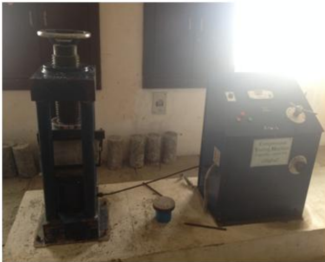
Fig 3.1.1 Compression testing machine (CTM)
