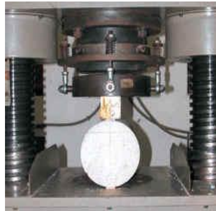
Testing of cylinder by split tensile
