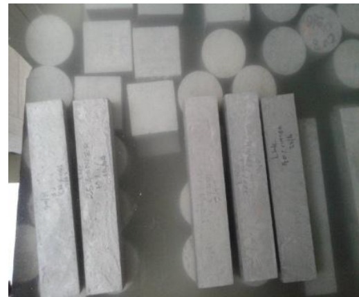
Curing of specimens
