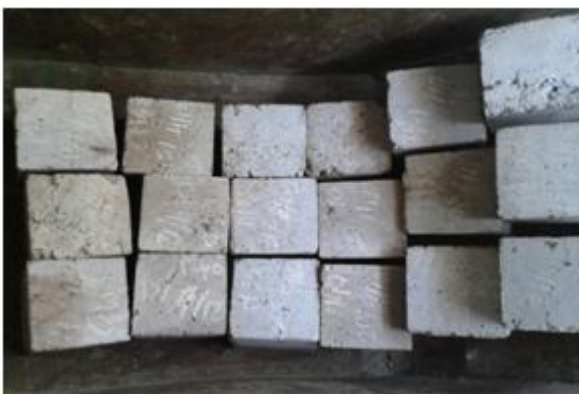
Cracks formed after cubes exposed to 8000c.
