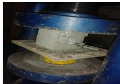
Cube under Compression Testing Machine after exposed to 2000c
