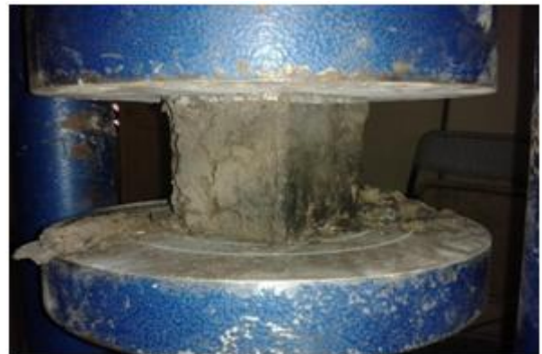
Failure of cube that is exposed to 8000c in compression testing machine
