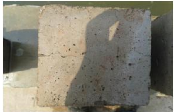
Cracks formed after cubes exposed to 8000c after cooled in water
