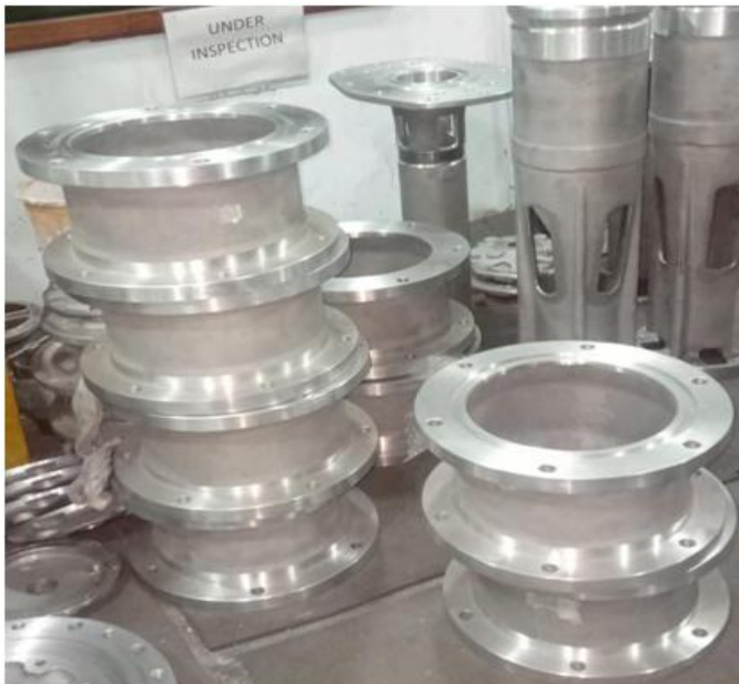
Figure 9: Component in production after Die modification
