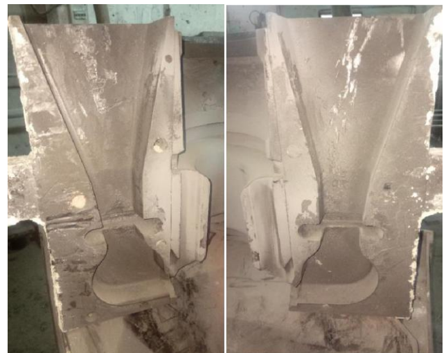
Figure 6: Both left and Right Dies after installation of new gating system
