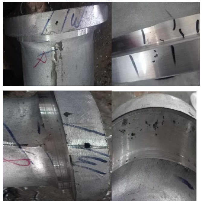
Figure 3: Various defects occurring due to Improper Gating Design
