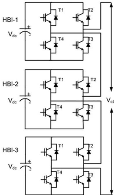
Fig. 2 Seven-level cascade inverter.
