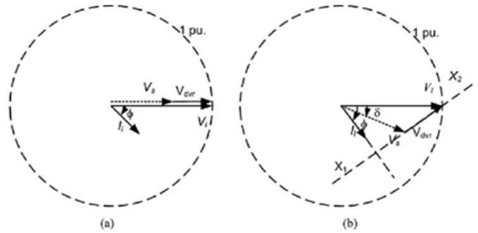
Fig. 4. Vector diagram for compensation of sag. (a) Inphase injection. (b) Zero active power injection.
