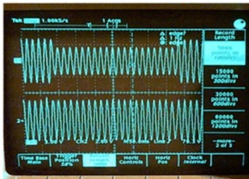
**Fig. 15. Experimental results for 12-cycles 40% supply voltage sag and mitigate load voltage waveforms.**
