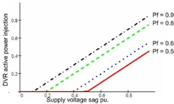
Fig. 7. Injected DVR active power versus the voltage sag for four different power factors.
