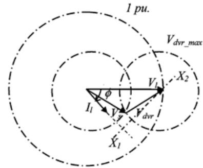
Fig. 6. Minimum real power injection with  $V_{dvr\_max} = 0.6$  p.u.
