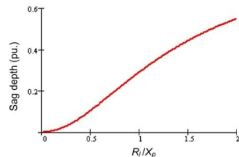
Fig. 9. Sag depth which can be mitigated without injecting real power for a different  $R_l=X_p$  ratio.
