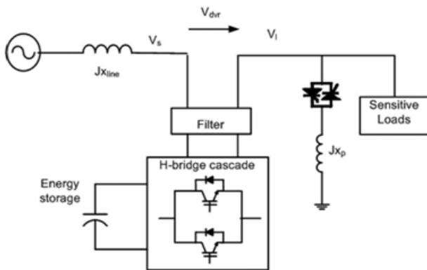
Fig. 3 Schematic diagram of a proposed new DVR.
