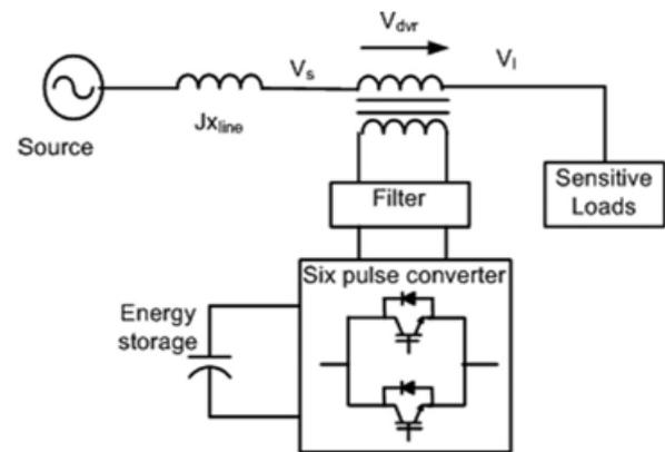
Fig. 1. Schematic diagram of a typical DVR
