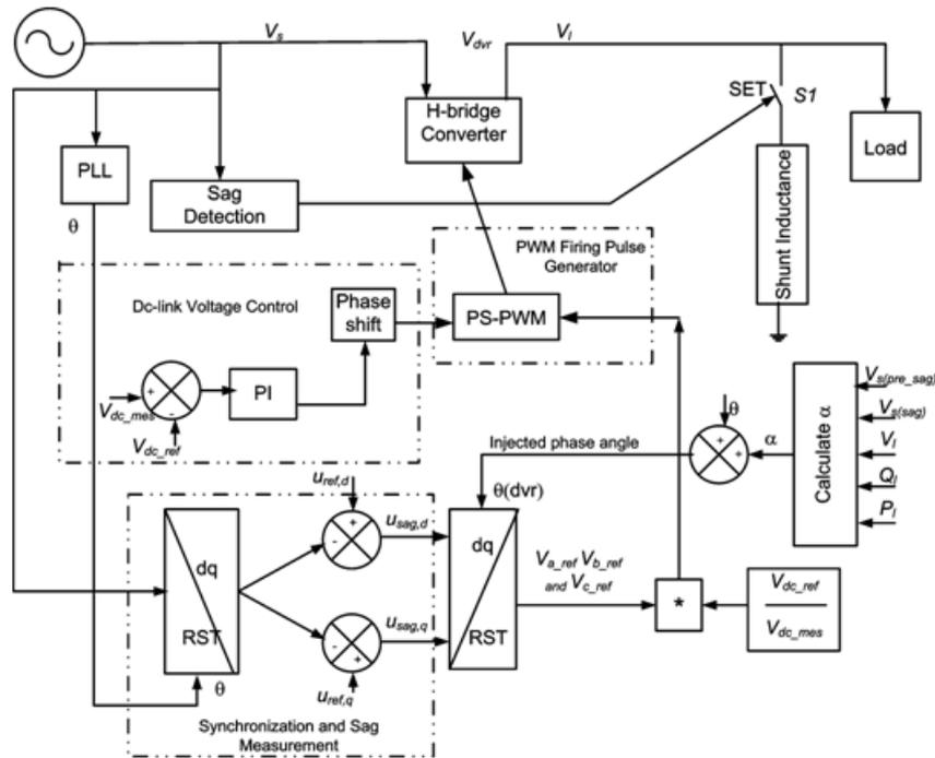
Fig. 10. Control structure of DVR with rotating dq reference.
