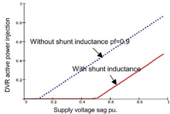
Fig. 8. DVR active power versus the voltage sag for the system without and with shunt inductance.
