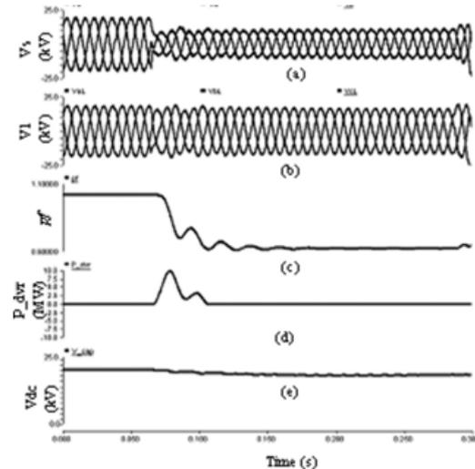
Fig. 13. Simulation results for the proposed DVR configuration for 40% seven-cycle sag correction with ( $R_l=X_p = 1.3$ ).
