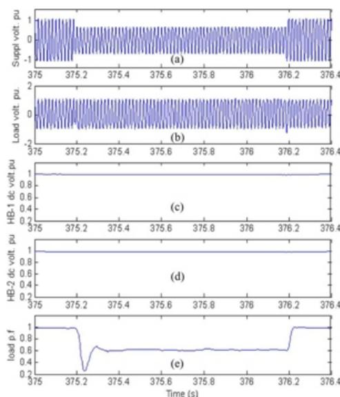
**Fig. 16. Experimental results for compensation of a 60-cycle 40% sag.**
