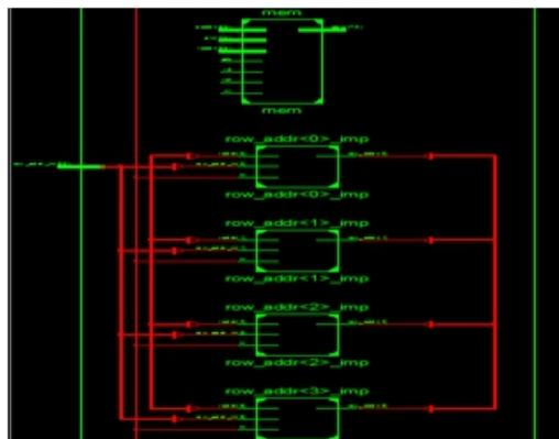
**Fig 8: Proposed RTL SCHEMATIC**
