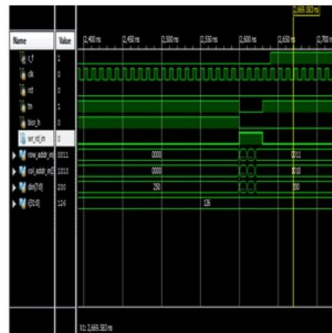
**Fig 11: Wave form of the error detected**
