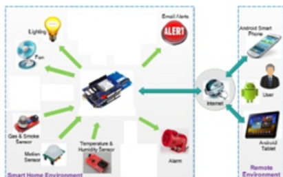
Fig. 1 Schematic image of a model home security system
