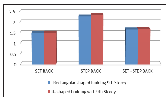
Figure 7 Max Time period for 9 th storeys Rectangular and U- shaped buildings with different configurations
