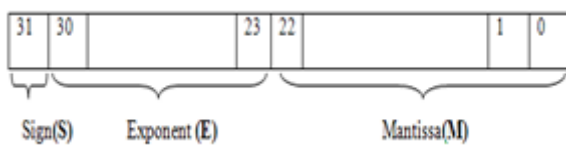
Fig.1 IEEE 754 single precision binary format representation
