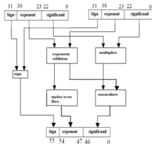
Fig 2 Block Diagram of floating point multiplier
