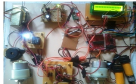
Figure-2: anti-collision and wiper speed control system.
