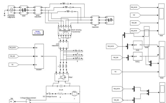
Fig.8. Matlab/Simulink Modelling of Proposed DVR under Voltage Sag/Swell Issues
