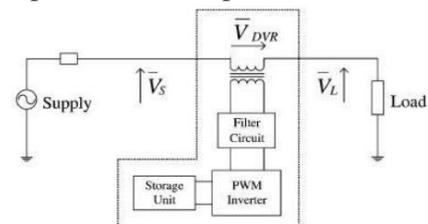
Fig.1: DVR series connected topology
