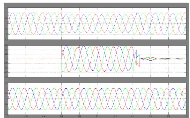
Fig.13. Source Voltage, DVR Injected Voltage, Load Voltage of Proposed DVR under Voltage Sag Issues
