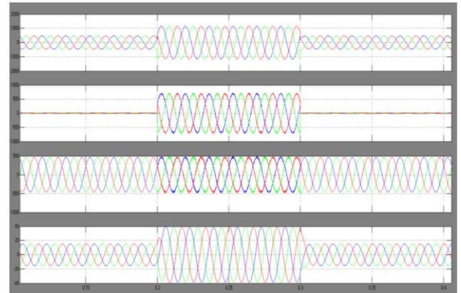
(a) Source Voltage, DVR Injected Voltage, Load Voltage, Source Current
