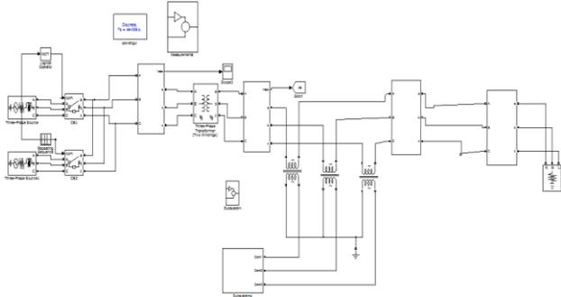
Fig.5. Matlab/Simulink Modelling of Conventional DVR under Voltage Sag/Swell Issues
