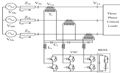
Fig. 3. Schematic of the DVR-connected system
