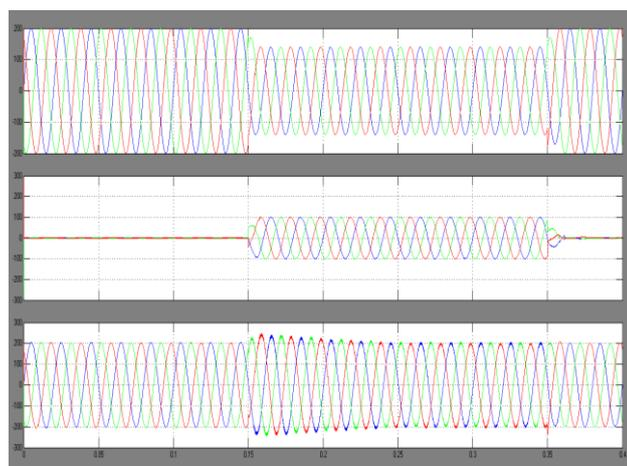
(b) Source Voltage, DVR Injected Voltage, Load Voltage
