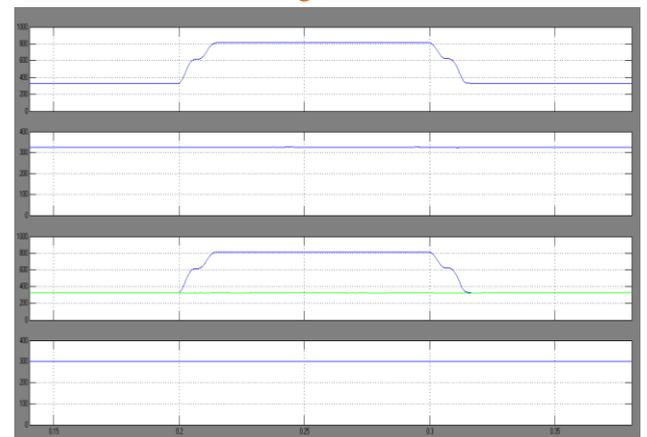
(b) RMS value of source voltage, load voltage, Its comparison, DC Link Voltage
