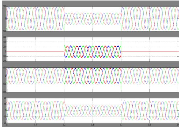
(a) Source Voltage, DVR Injected Voltage, Load Voltage, Source Current
