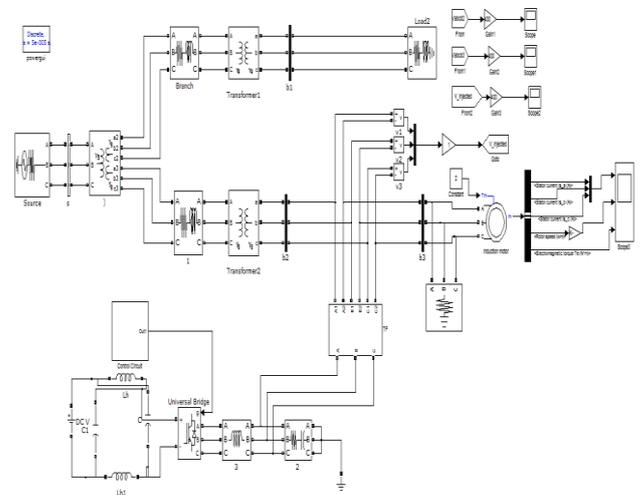
Fig.12 Matlab/Simulink Modelling of Proposed DVR under Voltage Sag/Swell Issues using Hysteresis Voltage Controller with induction motor drive
