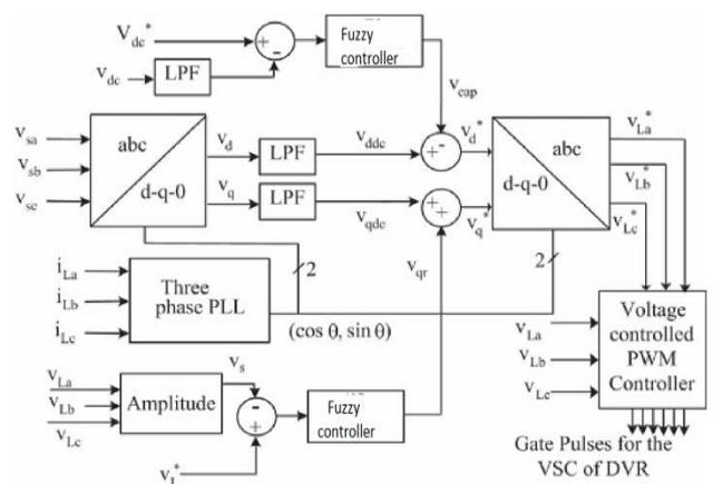
Fig. 4. Control block of the DVR that uses the SRF method of control
