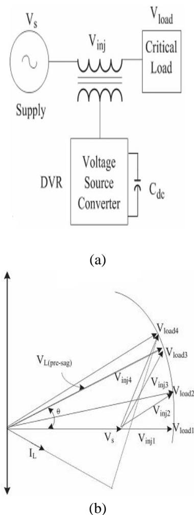
Fig. 2. (a) Basic circuit of DVR. (b) Phasor diagram of the DVR voltage injection schemes.
