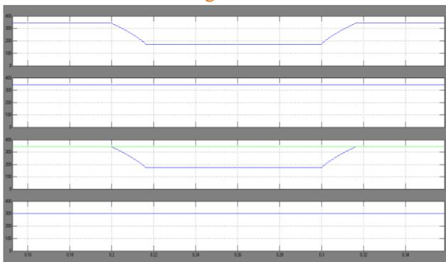
(b) RMS value of source voltage, load voltage, Its comparison, DC Link Voltage
