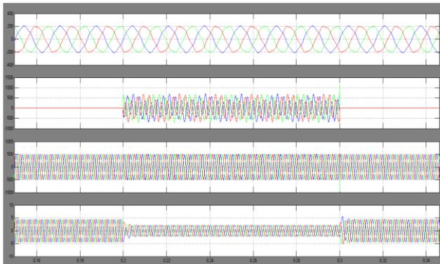
(a) Source Voltage, DVR Injected Voltage, Load Voltage, Source Current
