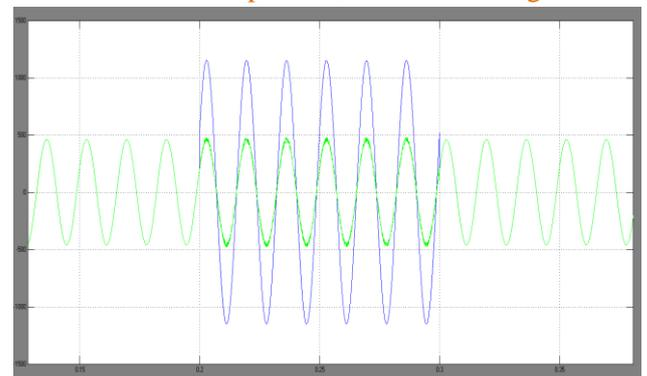
(c) Source Voltage & Load Voltage
