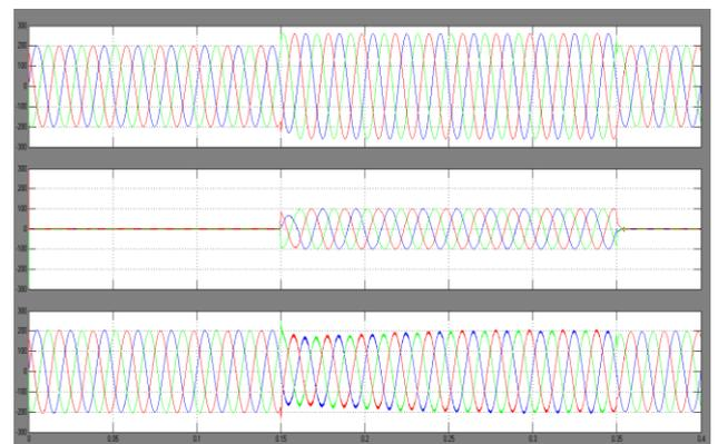
(b) Source Voltage, DVR Injected Voltage, Load Voltage
