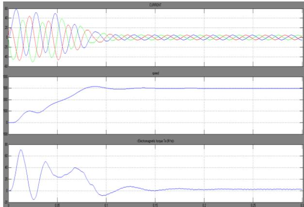
Fig.14.Simulation result for stator currents, speed and electromagnetic torque of induction motor
