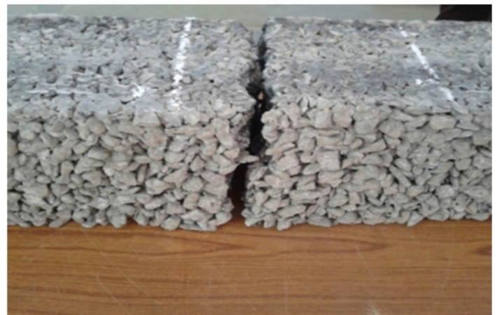
Fig.5: Beam failure after applying a load
