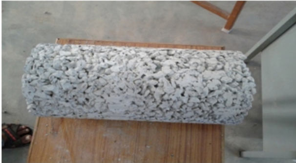
Fig.4: Cylindrical specimen is failed by applying tensile load along horizontal direction
