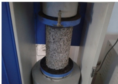
Fig.1:A cylindrical specimen is placing in the compression testing machine The cylindrical specimen is of the size 15mm*300mm.
