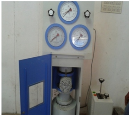
Fig.2: A cylindrical specimen placing in horizontal direction in the machine
