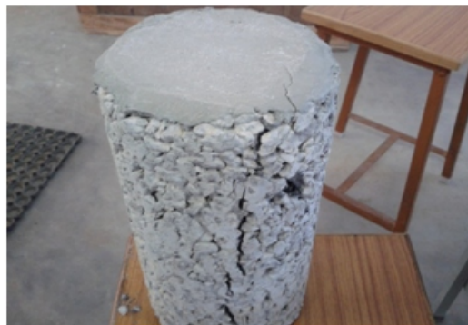
Fig.3: Cylindrical specimen after the failure of applied compressive load
