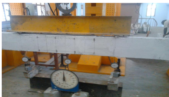
Fig 2, Normal Re beam where tested under four-point load
