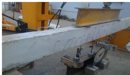
Fig3: Bonded GFRP beam where tested under four-point load
