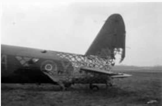
Fig 3.2 Geodesic airframe fuselage structure is exposed by battle damage
