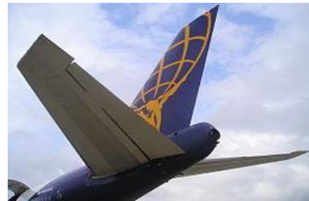
Fig 1.3 The empennage of a Boeing 747-200
