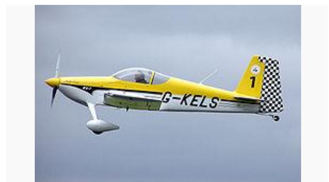
Fig 3.3 The Van's Aircraft RV-7 fuselage is slender for high speed flight
