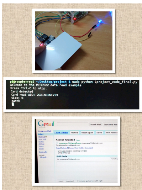
Figure 5: A snapshot of NFC card ‘match’ condition
