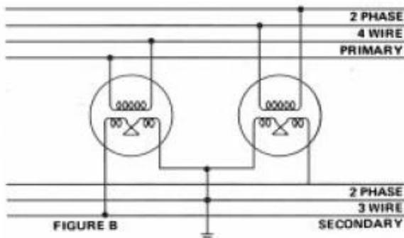
Fig.11. represents a two-phase system is simply two single-phase circuits
