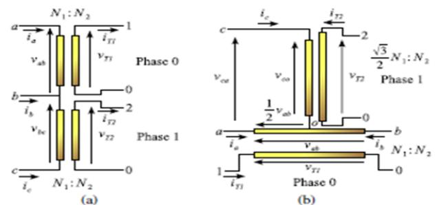
Fig. 1 Traction transformer schemes. (a) V-V transformer. (b) Scott transformer
