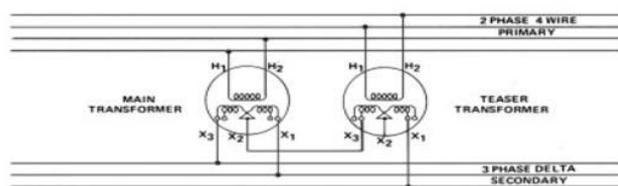
Fig .26. Represents Scott Connection Three-Phase to Three-Phase
