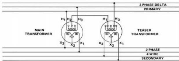
Fig.25. Represents Scott Connection Three-Phase to Two-Phase
