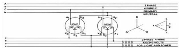
Fig.22. Represents Y-Delta With One Unit Missing
