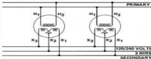
Transformer is placed between high-voltage line and low voltage. The 120/240-volt low-voltage windings are connected in parallel. This type of connection would be used to supply one customer with 120 volts for lights.
