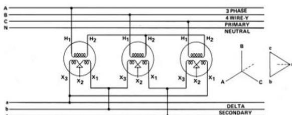
Fig.20 Represents Y-Delta for Power 210 degrees out phase with angular displacement
