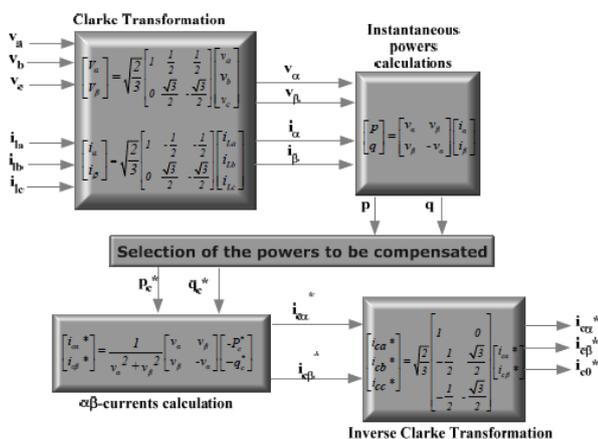
Fig. 31. Control method for Shunt current compensation based on p-q theory
