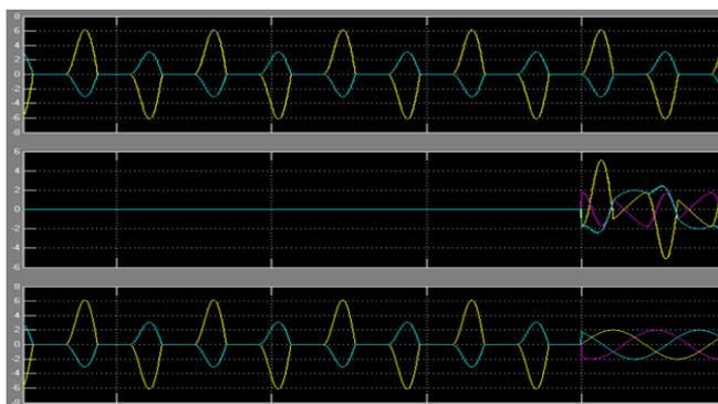
Figs .35 represent Scott connection uncompensated, filter& compensated currents
