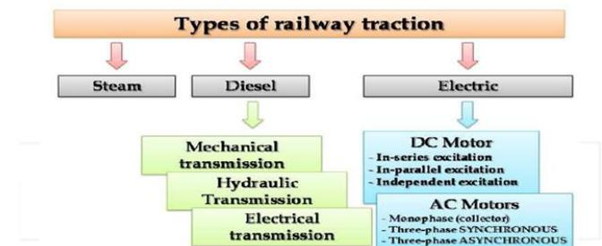
Fig 7. represents railway engine and motor types
