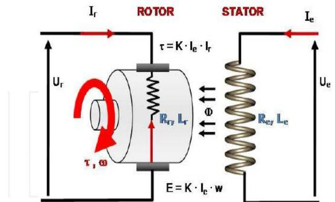
Fig. 9. Electromechanical circuit diagram of a DC electric motor.
