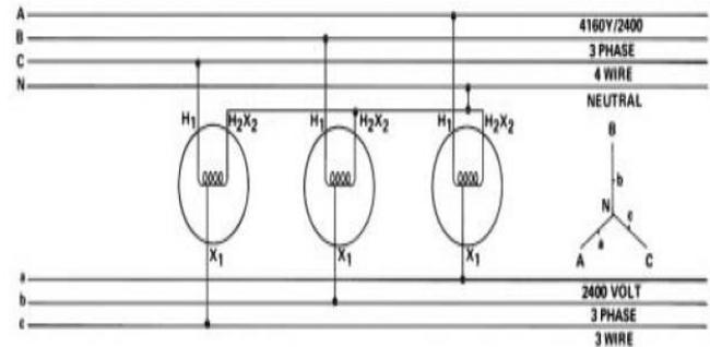
Fig .24. Represents Y-Y Autotransformers for Supplying Power to 2400-Volt Motors from a 2400/4160Y-Volt Three-phase Four-Wire System
