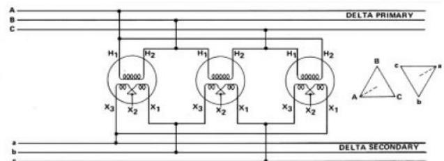
Fig.13. represents Delta-Delta for Power 180 deg out phase
