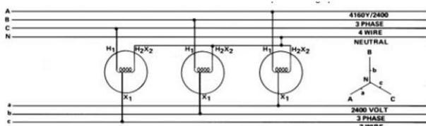
Fig.10. Represents three-phase delta banks connected to 2400/4160Y-volt systems
