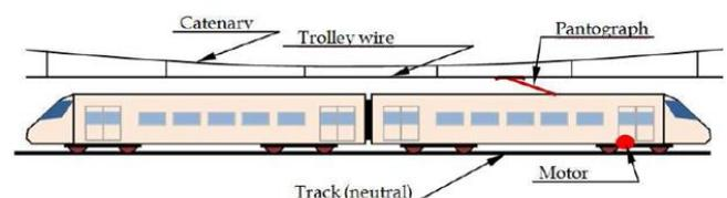
Fig 8. Electric railway traction: General outline, catenary and pantograph.
