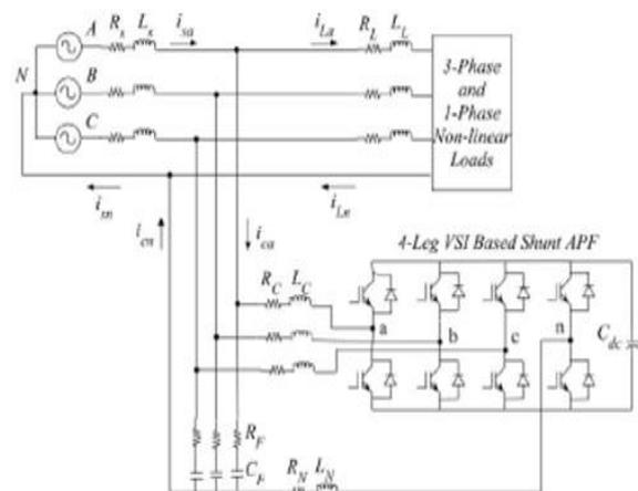
Fig .28. Four-leg shunt APF with non-linear load
