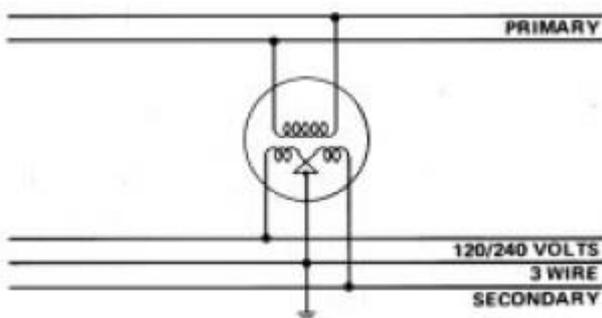
For Power This connection is similar to single phase for lights except 120/240-volt low-voltage windings are hooked in series giving 240 volts on a two-wire system as shown
