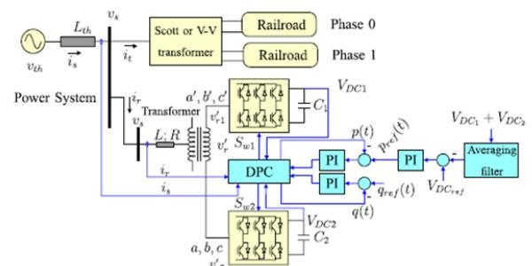
Fig 3. Proposed compensation scheme
