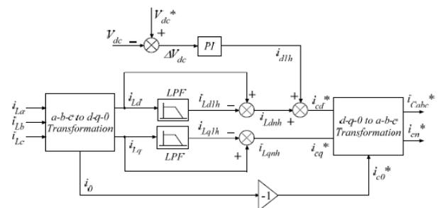
Fig .30. Reference current extraction with  $id-iq$  method
