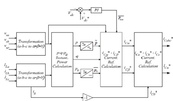
Fig .29.. Reference current extraction with conventional  $p-q$  method
