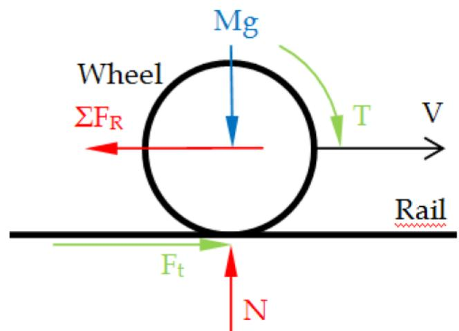
Fig 5 represents Tangential adhesion forces in the wheel-rail contact
