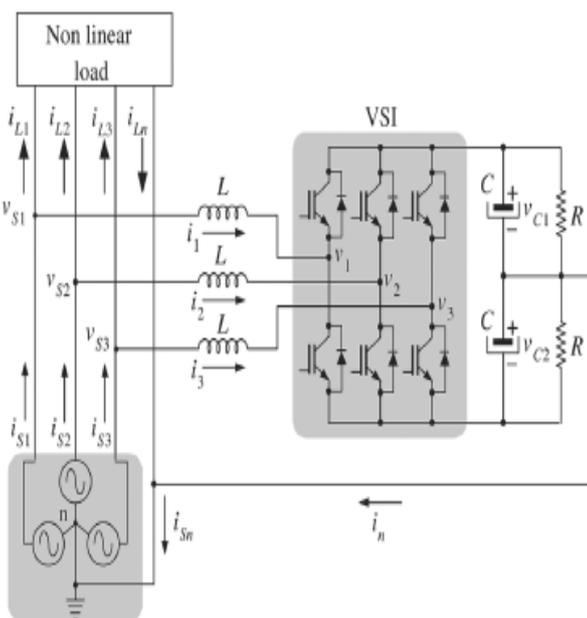
Fig .27. Three-leg shunt APF with non-linear load
