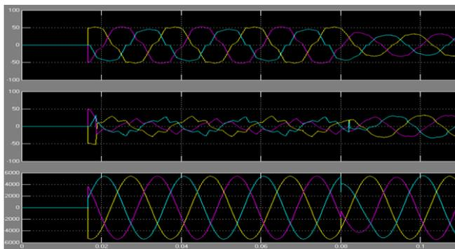
Fig .33 represents simulated waveforms for the Scott transformer connection for different Railroad load profiles
