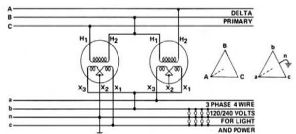
Fig 18. Represents Open Delta for Light and Power
