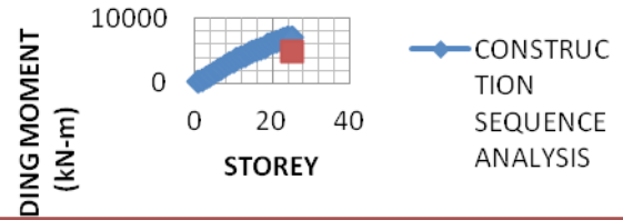
Fig. 10: BENDING MOMENT OF TB2 WITH CONSTRUCTION SEQUENCE ANALYSIS
