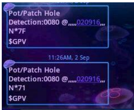
Fig.4. Message sent to android device about the pothole locations
