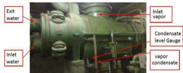
Fig 4.1: Condenser setup in industry
