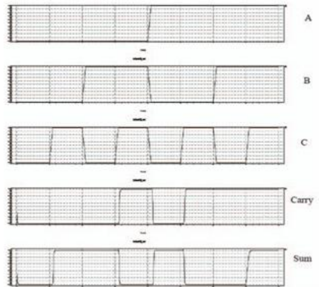
FIG. 6. 2T GDI BASED 2:1 MUX TRANSIENT RESPONSE.
