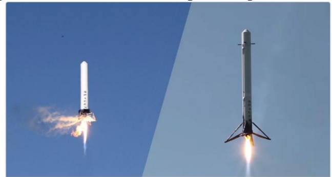
Fig 1.2:- Grasshopper, left, and the F9R-Dev1, right. The diameter of the two is identical.
