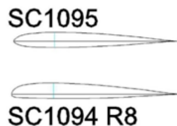
Fig 3.3 Chord length and Maximum thickness of airfoils at each stations are noted.
