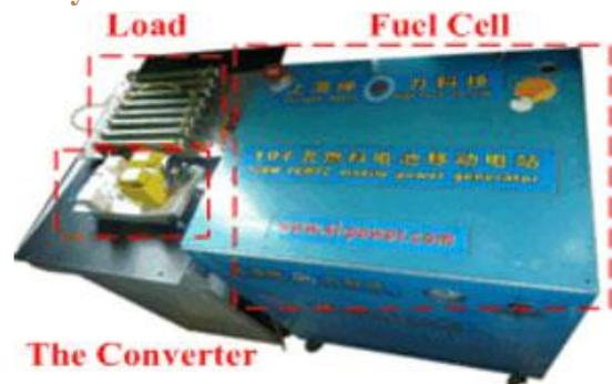
Fig. 11. Prototype of the 1-kW Converter with fuel cell and load.
