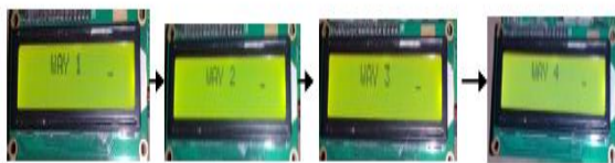
Fig 15: Showing 4 ways one by one on LCD display when there is no traffic
