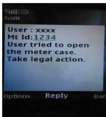
Fig 5: Message Received When User Tried to Open the Meter Case
