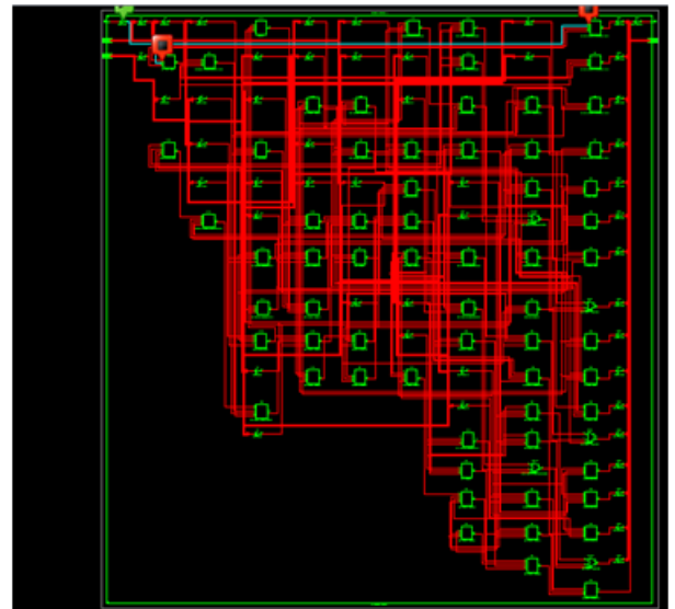
Fig9: Technology Schematic of 16bit-BK-BEC Carry select adder
