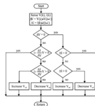
Fig: 2.6 perturb & observe algorithm with voltage reference
