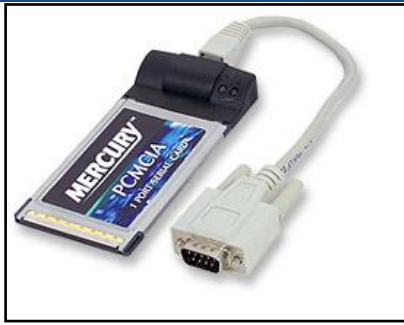
Figure 5 PCMCIA to RS232 Adapter
