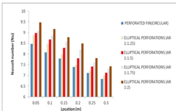
**Fig 4.9: Local Nusselt number distribution for circular and elliptical perforated fins along the flow direction**
