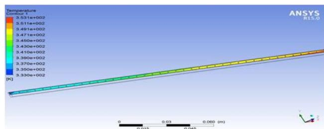
**Fig 4.6: Temperature Contour for Circular Perforated Fin**
