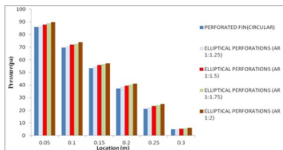
**Fig 4.7: pressure distribution for circular and elliptical perforated fins along the flow direction.**
