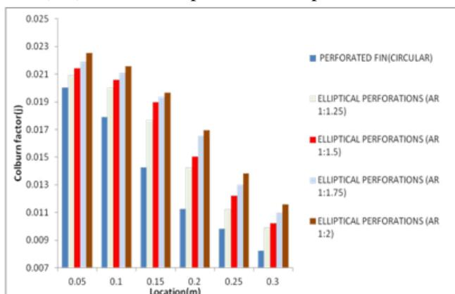
**Fig 4.10: Local Colburn factor distribution for circular and elliptical perforated fins along the flow direction.**
