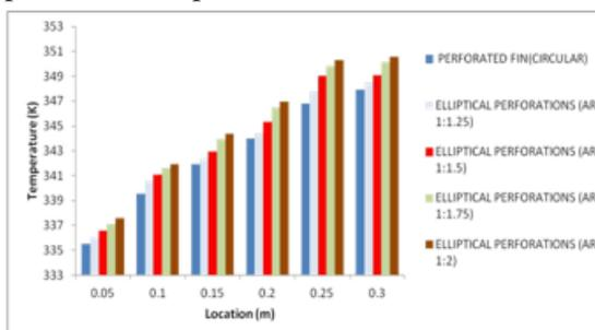
**Fig 4.8: Temperature distribution for circular and elliptical perforated fins along the flow direction.**
