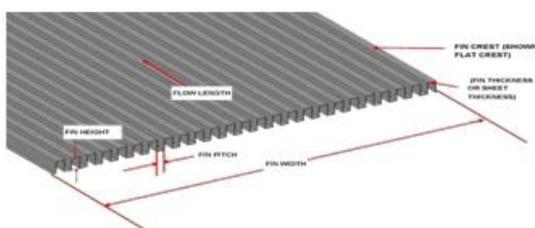
**Fig 3.1: Plain fin Heat Exchanger**
