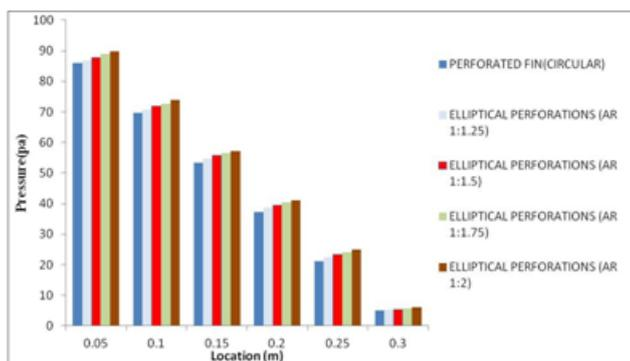
Fig 6.2: Comparison of pressure distribution for circular perforation and elliptical perforated fin along the direction of flow
