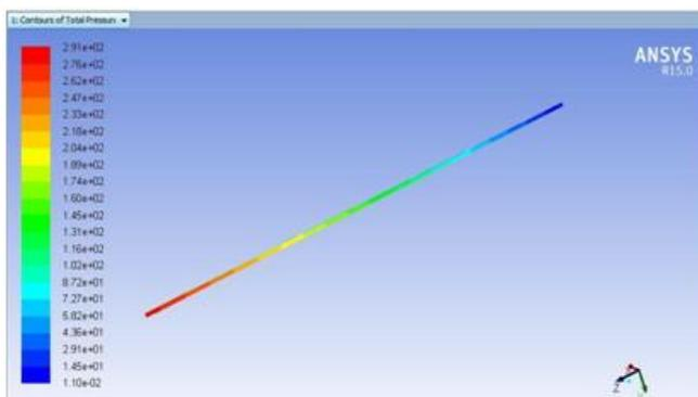
Fig 3.6: Pressures Contour for Plain Fin
