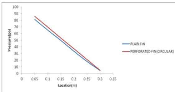
Fig 6.1: Comparison of pressure distribution for plain fin and circular perforated fin along the direction of flow
