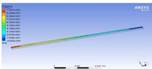
**Fig 4.5: Pressures Contour for Circular Perforated Fin**
