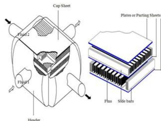
**Fig 1.1: Plate fin heat exchanger**
