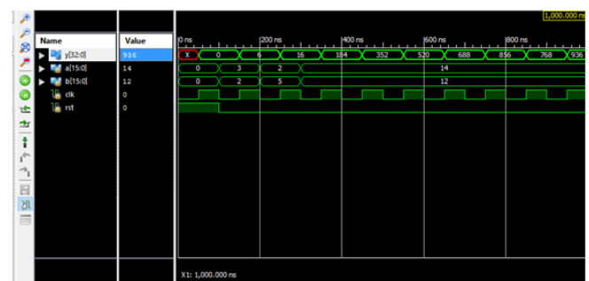
Fig. 13. Simulation of MAC unit CI-CSKA
