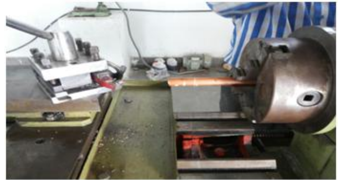
Turning copper cylindrical rod
